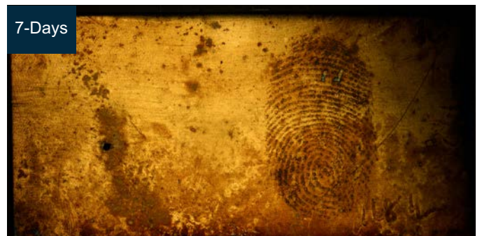
A brass plate seeded with fingermarks and washed with dilute bleach before being treated using the RECOVER technique.
